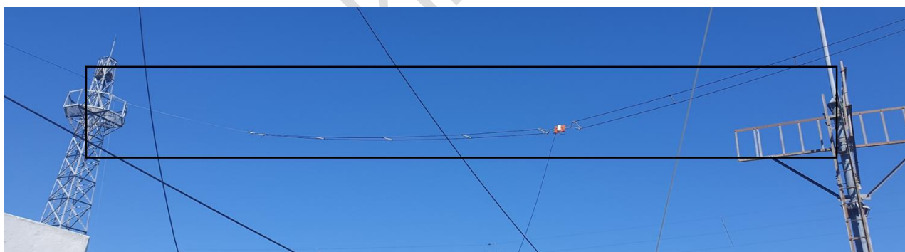
Figure 5 Digital HF Receiving Antenna Prototype
