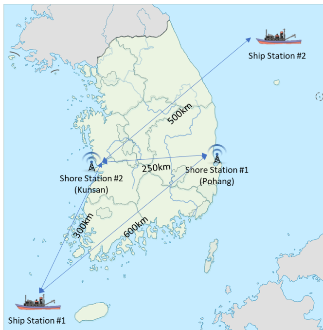
Figure 6 Digital HF testbed plan in Korea
